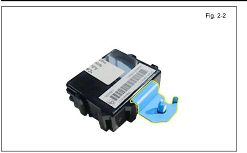
b. Attach the GBS ECU Bracket to the GBS ECU as shown.
